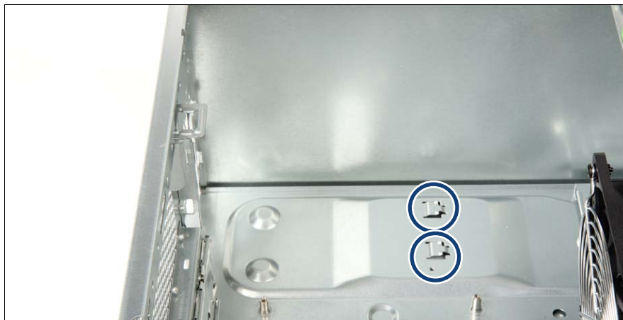
Figure 38: Hooks for fastening the PSU
