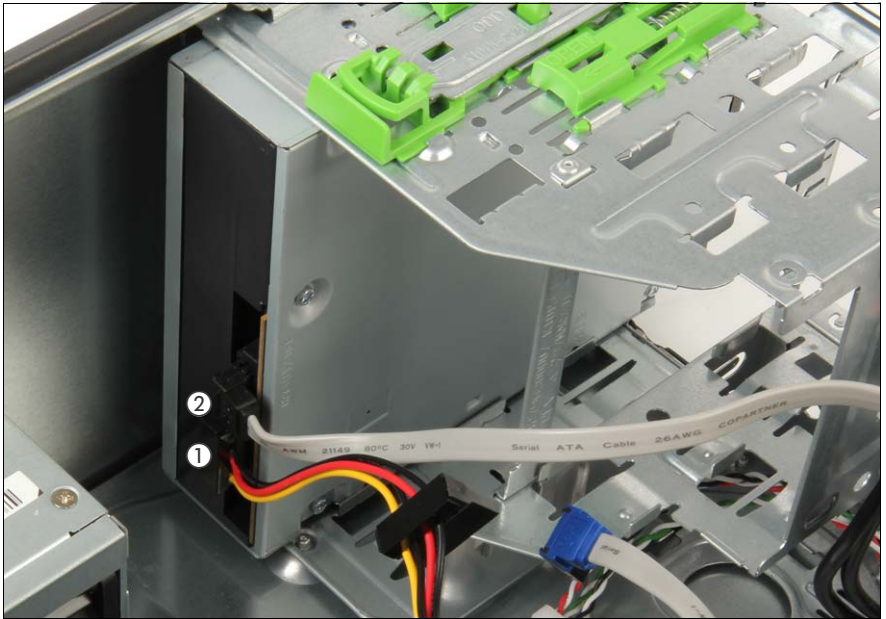
Figure 150: Connecting cables to the optical disk drive
