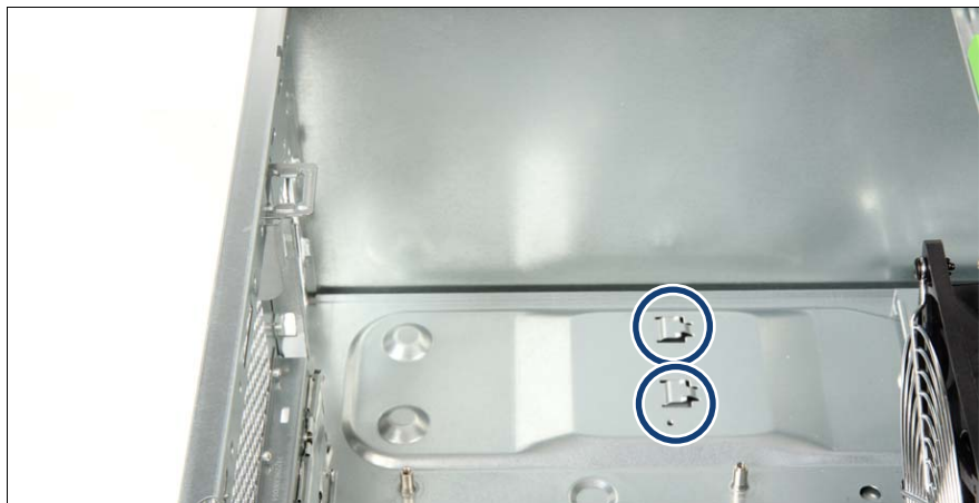
Figure 30: Hooks for fastening the PSU
