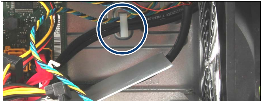
Figure 64: Cable clamp of the fan cable
