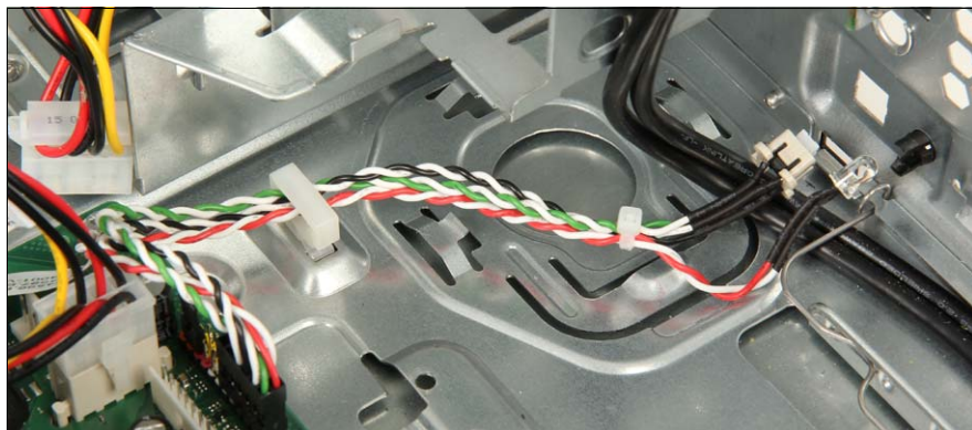
Figure 184: On/Off button and LED removed
