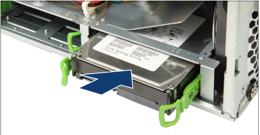
Figure 47: Inserting the 3.5-inch HDD
