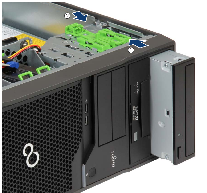
Figure 7: Removing the optical disk drive
