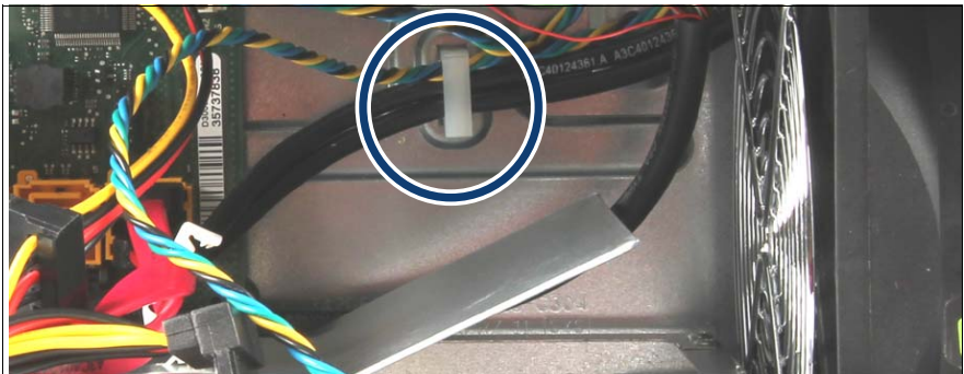
Figure 69: Cable clamp of the fan cable
