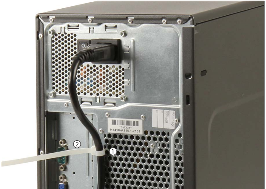
Figure 17: Securing the power cord
