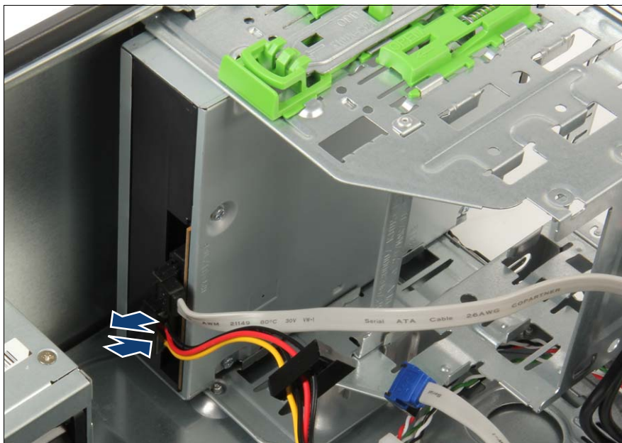
Figure 226: Disconnecting/connecting power cable on the optical disk drive
