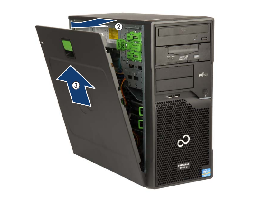
Figure 5: Removing the side cover
