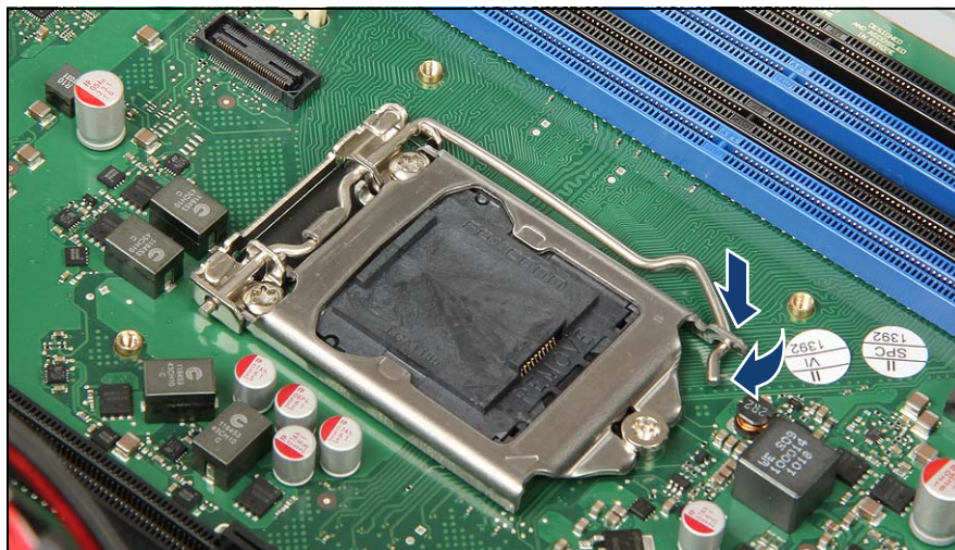
Figure 218: Installing the protective socket cover (defective system board) (C)
