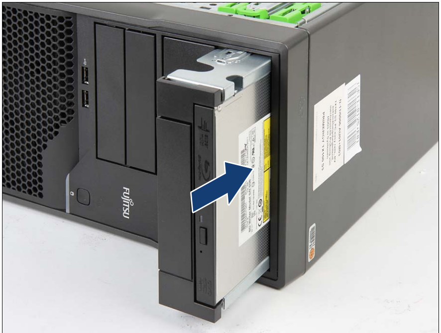
Figure 157: Installing the slide-in unit
