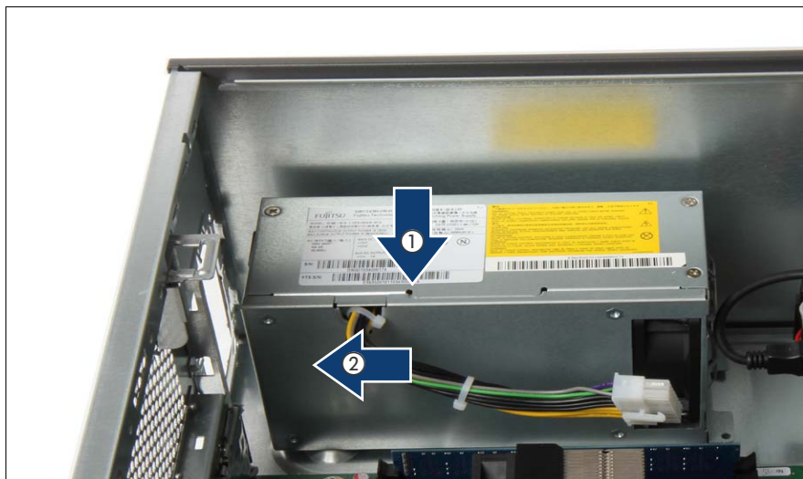
Figure 31: Installing the PSU
