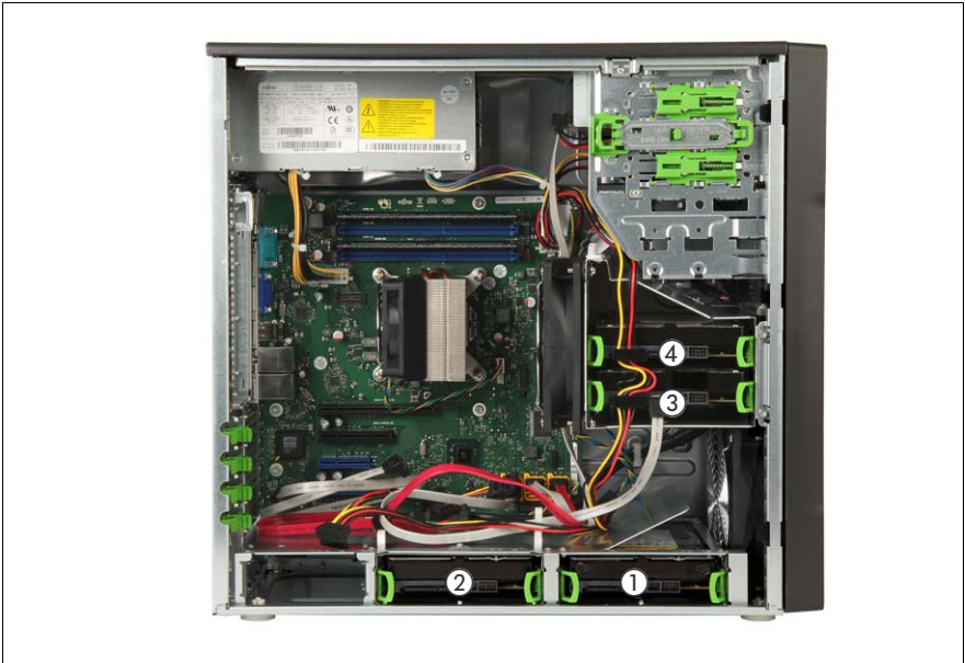
Figure 43: 3.5-inch HDD mounting order
