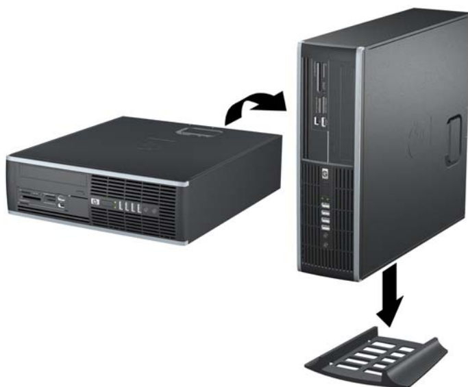
Figure 2-6 Changing from Desktop to Tower Orientation
