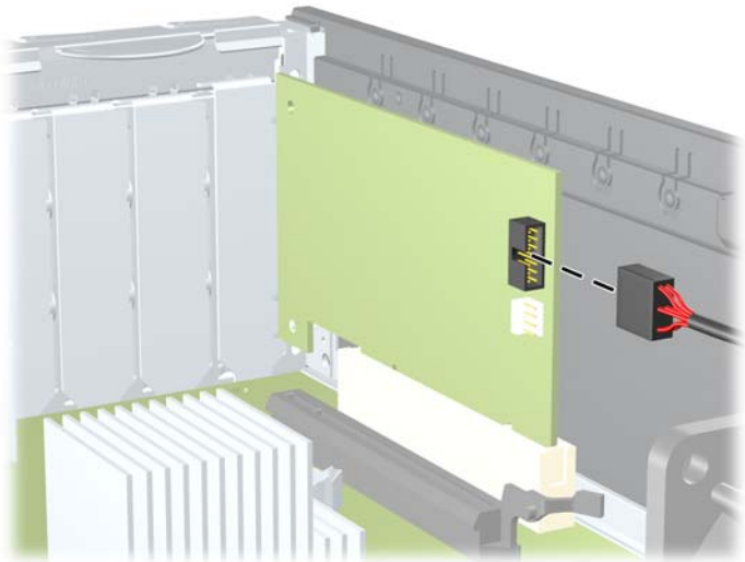
Figure 2-30 Disconnecting the Media Card Reader 1394 Cable
