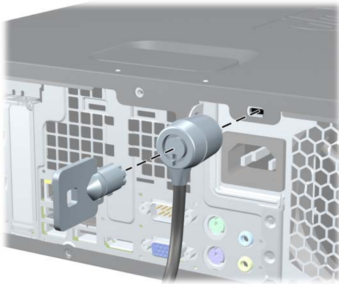
Figure C-1 Installing a Cable Lock
