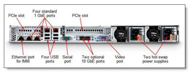
Figure 3. Rear view of the IBM System x3550 M4
