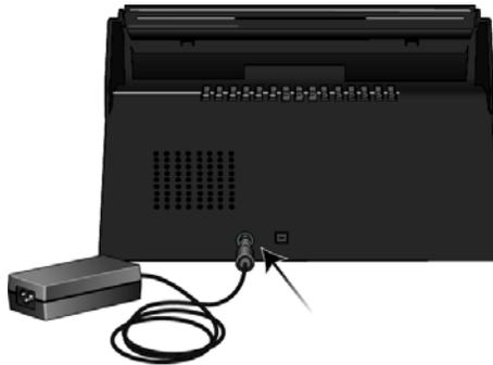
**Note:** Only use the power supply (HEG42-240200-7L made by HiTron) included with your scanner. Connecting any other type of power supply may damage your scanner, and will void its warranty.
