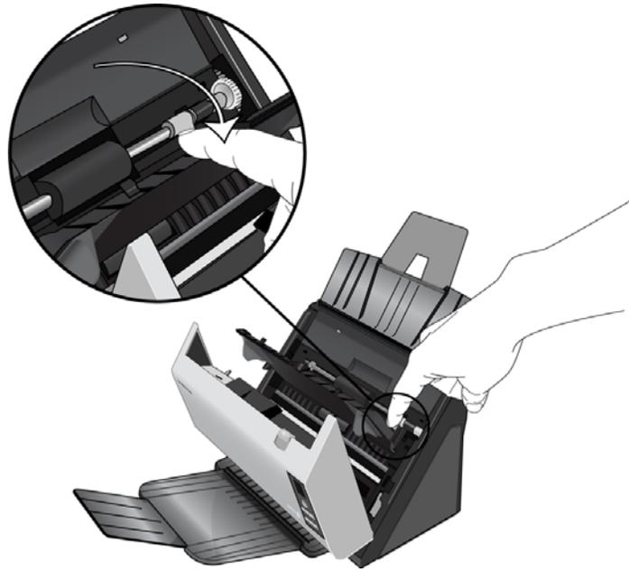
10. Lift the paper guide up to the back of the scanner and press gently on the paper guide until it snaps into place.
