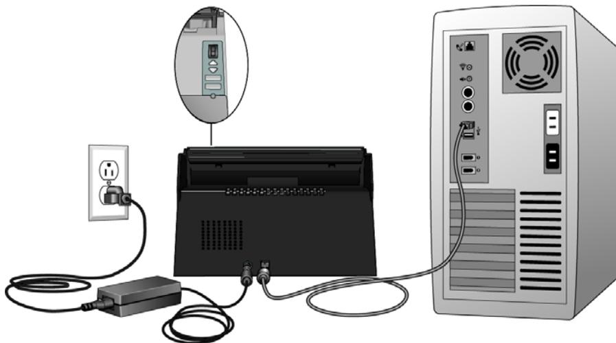
The status light comes on and flashes indicating that the scanner is receiving power. Your computer recognizes that a scanner has been plugged into the USB port and automatically loads the appropriate software to run the scanner. If your computer is running Windows version XP or later, you will see a message similar to the one below.
