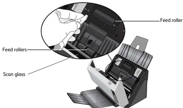
4. Wipe clean the free rollers, ADF pad, and scanner glass in the under side of the ADF door. Be careful not to snag the cloth on the spring arms of the ADF pad.
