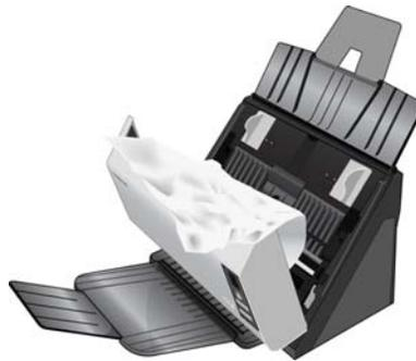
To reduce the number of paper jams, smooth and straighten the paper before scanning, adjust the guides to the paper size, and insert the paper evenly into the ADF
