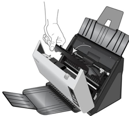
4. The roller is held in place with a lock tab that rotates to lock and unlock it. To unlock the tab, rotate it upward until the small lock flange is completely free.
