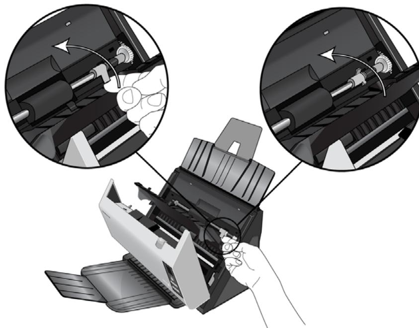
5. Remove the roller from the scanner and discard it, it cannot be repaired.
