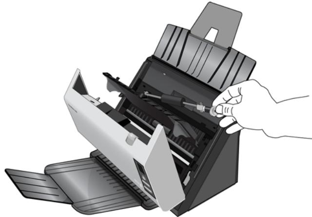
8. Angle the roller into the scanner and align the lock tab with the slot in the scanner.
