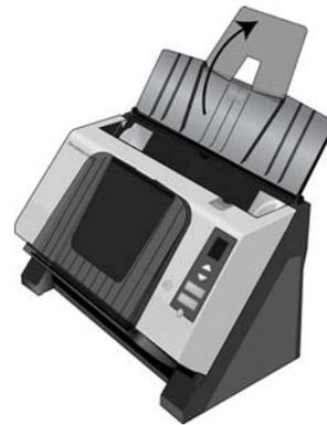
4. Pull the output tray down from the scanner body. It will snap in place when it is down all the way. Make sure the bottom of the tray is down all the way before scanning. If the tray isn't fully seated in position, paper feeding from the input tray may jam in the scanner.
