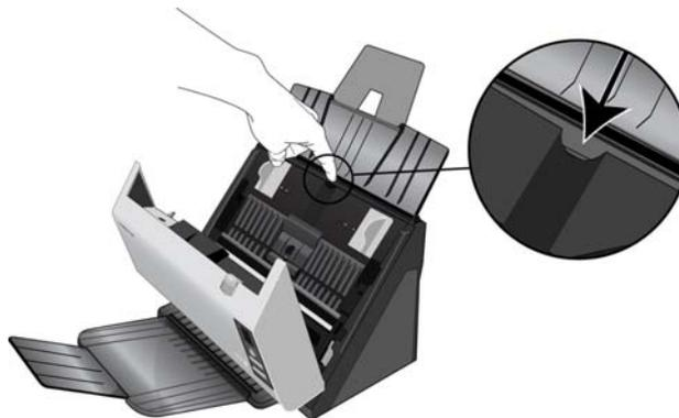
3. The replaceable roller is located behind the paper guides.
