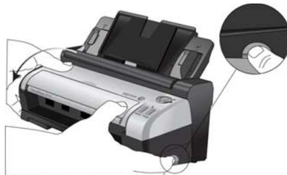
2. Tilt the scanner body towards the front of the Docking Station to release the scanner from the arms in the Docking Station.
