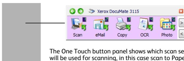
The One Touch button panel shows which scan setting will be used for scanning, in this case scan to PaperPort.
