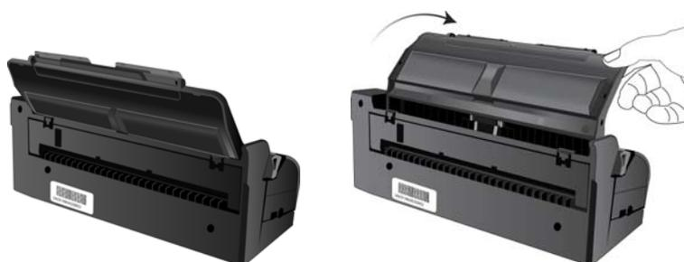
2. Press down on the two latches on the back of the docking station and lower the rear cover.
