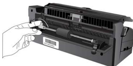
4. When the roller is unlocked, it can be removed from its mounting sockets.
