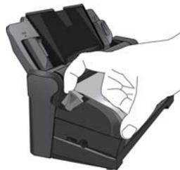
3. Wipe the scanner glass and plastic surfaces on the inside of the scanner. Make sure you clean the glass located in the scanner body and on the underside of the scanner lid. Be careful not to snag the cloth on any of the surfaces inside the scanner.
