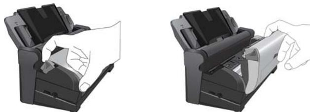
5. Detach the scanner body from the docking station and remove the foam strip from the docking station.
