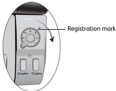
2. Place an item *face down*, on the front feed tray, aligned to the registration marks on the tray and insert it into the front of the scanner.
