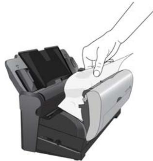
To reduce the number of paper jams, smooth and straighten the paper before scanning and adjust the guides to the paper size, and insert the paper evenly into the ADF.
