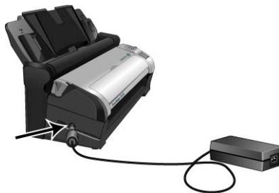
**NOTE:** Only use the power supply (either HEG42-240100-7L made by HiTron or DA-24C24 made by ADP) included with your scanner. Connecting any other type of power supply may damage your scanner, and will void its warranty.
