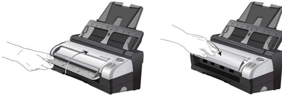
1. Adjust the paper guide for the width of paper, and make sure the input and output trays are fully extended.
