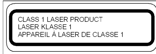
Example of Class 1 Laser Warning Label
