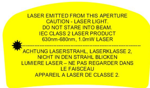
Example of Class 2 Laser Warning Label
