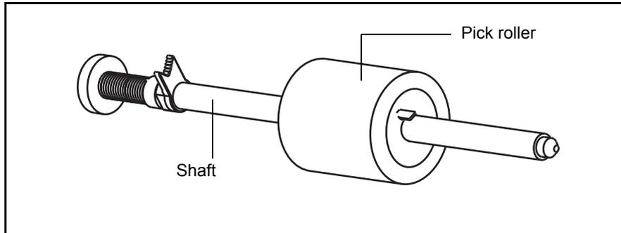
Replace the pick roller following the procedure below.
