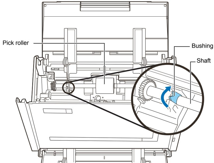
**6. Remove the pick roller with its shaft.**
