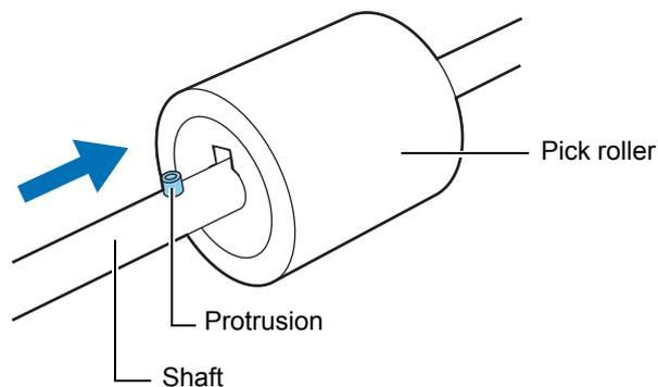
**9. Install the pick roller with its shaft to the ScanSnap.**
