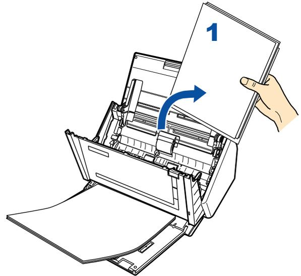
2. Remove documents to be re-scanned (2) (normally two sheets or more) from the stacker, and reload in the ADF paper chute (cover) without changing the direction in which the documents are facing.
