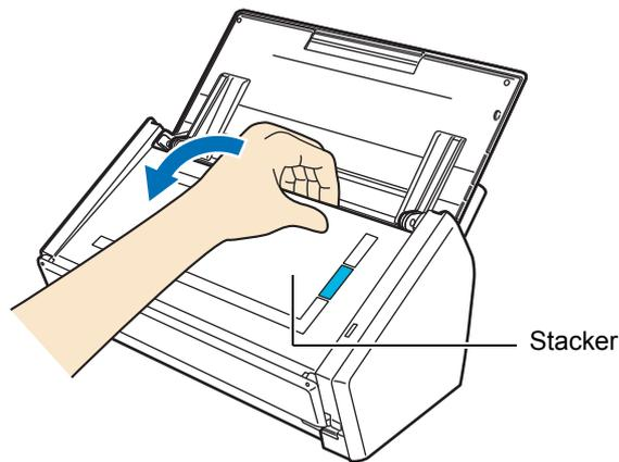
**6. Pull out the extension of the ADF paper chute (cover), and open the stacker.**
