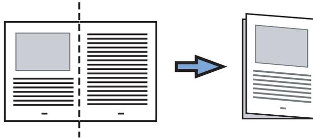
2. Open the Carrier Sheet and insert the document. Align the fold with the right edge of the Carrier Sheet so that the document fits into the Carrier Sheet at the upper corner.
