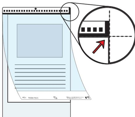
3. Load the Carrier Sheet into the ScanSnap.
