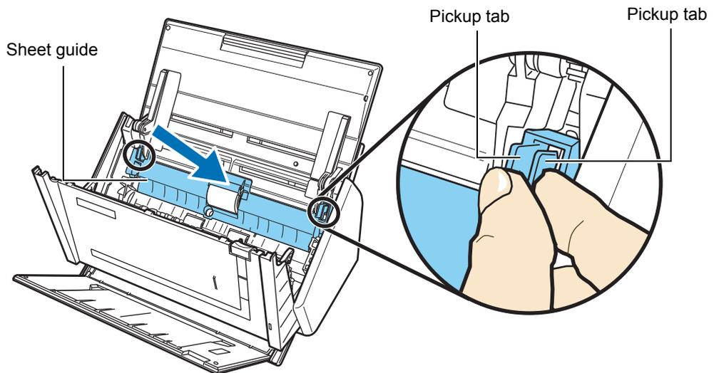
⇒ The sheet guide makes a clicking sound when the pickup tabs fix into position.
