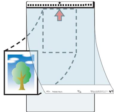
2. Load the Carrier Sheet into the ScanSnap.
