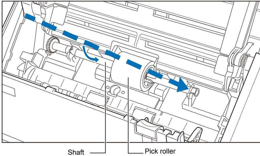
**10. Secure the bushing (left) by rotating it in the direction of the arrow.**
