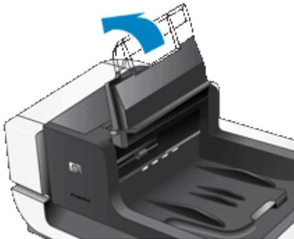
2. Lift the green lever slightly, and then slide the imprinter to the position that you want.
