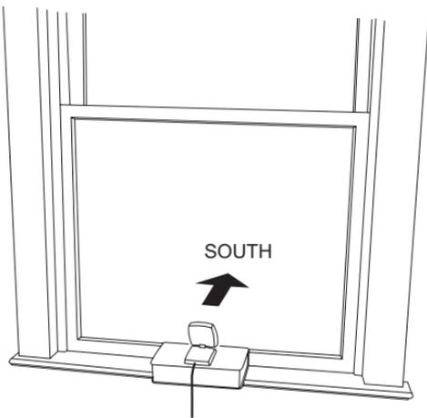
you receive a consistent signal, or placing the antenna in a window is not a practical solution for you, **BETTER** reception can be achieved by placing the antenna outside on a window ledge, porch, table, or patio. The location you choose should provide the antenna with a clear view of the southern sky.
