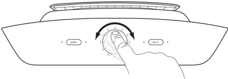
The audio can be muted by pressing the volume control twice. The outer circle of blue lights will blink to indicate the Radio is muted. Press twice again to un-mute the Radio.
