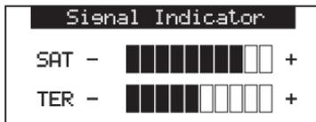
Refer to your radio's User Guide for instructions, and access the **Signal Indicator** or **Antenna Aiming** screen of your radio to see a visual indication of signal strength. If you're receiving good Satellite and Terrestrial signal strength, you're done. If not, try some of the suggestions which follow.
