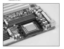
5. Connect the power wire to a power source on your motherboard.
