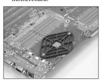
4. Hook the clip to the retention plate from one side.
