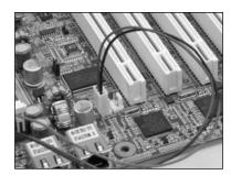
2. Attach the diamond-shaped plastic plate to the bottom of the motherboard.
