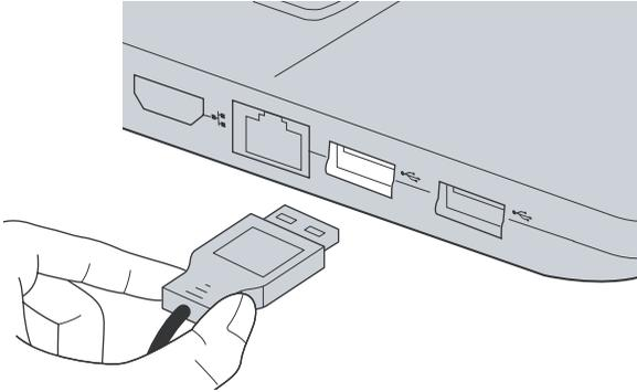
The first time you plug a USB device into a particular USB port on your computer, Windows automatically installs a driver for that device. After the driver is installed, you can disconnect and reconnect the device without performing any additional steps.
