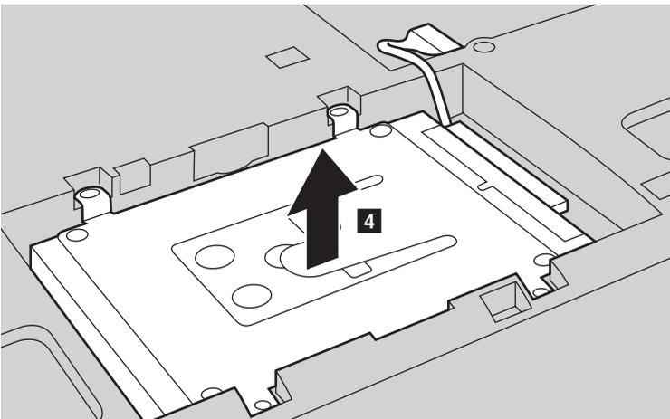
**Note:** Be sure to remove the hard disk (secured in the metal frame) gently to avoid breaking the connection to the SATA receptacle connector.
