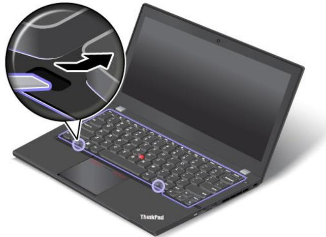
4. Loosen the screws that secure the keyboard with the keyboard multi-tool.
