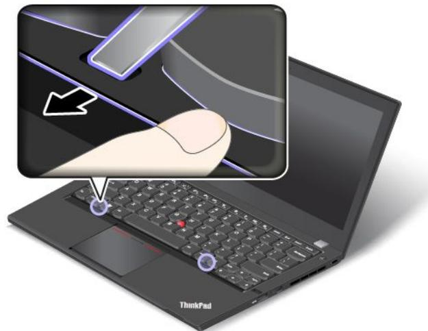
6. Adjust the keyboard frame in place with the keyboard multi-tool and ensure that all the latches are secured under the keyboard bezel.
