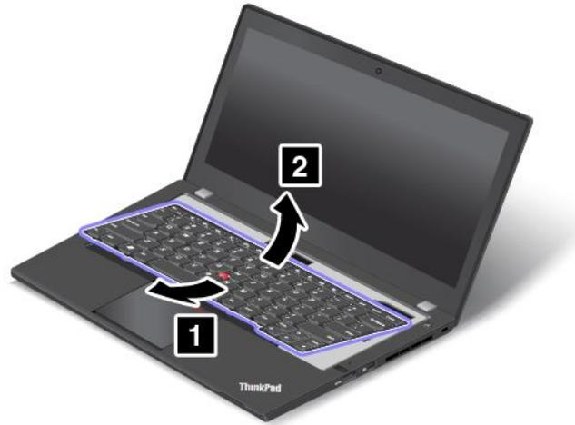
6. Put the keyboard on the palm rest and detach the connectors. Then remove the keyboard.
