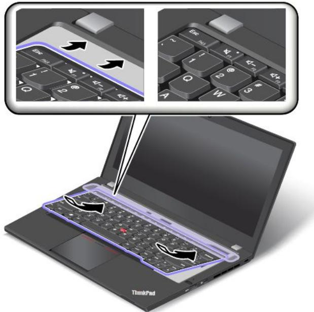
3. Ensure that the screw heads are exposed completely. Otherwise, reveal the screw heads by sliding the keyboard frame forward with the keyboard multi-tool.
