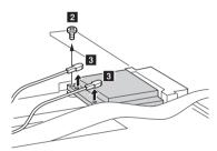
In step **2**, unplug the jacks by using the removal tool antenna RF connector (P/N: 08K7159), or pick up the connectors with your fingers and gently unplug them in the direction shown by arrows.
