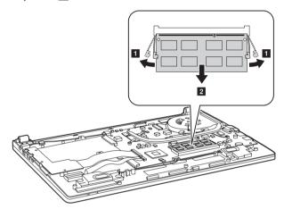
**When installing:** Insert the notched end of the DIMM into the socket. Push the DIMM firmly, and pivot it until it snaps into the place. Make sure that it is firmly fixed in the slot and difficult to be moved.
