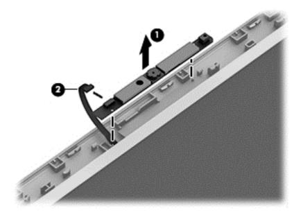
**c.** Remove the webcam/microphone module.
