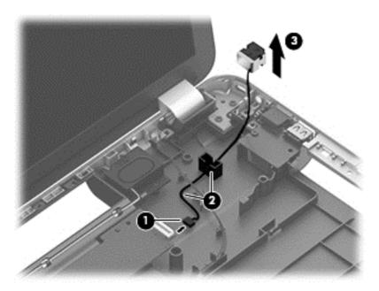
4. Remove the power connector cable.
