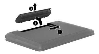
Reverse this procedure to install the battery.
