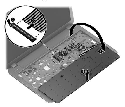
Reverse this procedure to install the keyboard.
