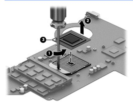
Reverse this procedure to install the processor.
