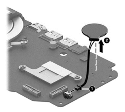
**4.** Remove the RTC battery.
