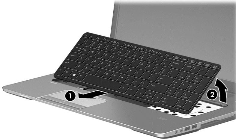
7. Rotate the keyboard until it rests on the palm rest **(1)**, and then disconnect the keyboard cable by lifting the keyboard connector latch **(2)**, and then disconnecting the keyboard cable from the system board **(3)**.
