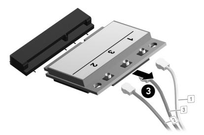
NOTE: WLAN modules are designed with a notch to prevent incorrect insertion.
