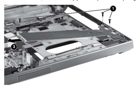
Reverse this procedure to install the audio/USB  $3.0\ board.$
