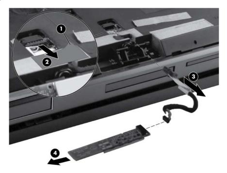
Reverse this procedure to install the Bluetooth module.
