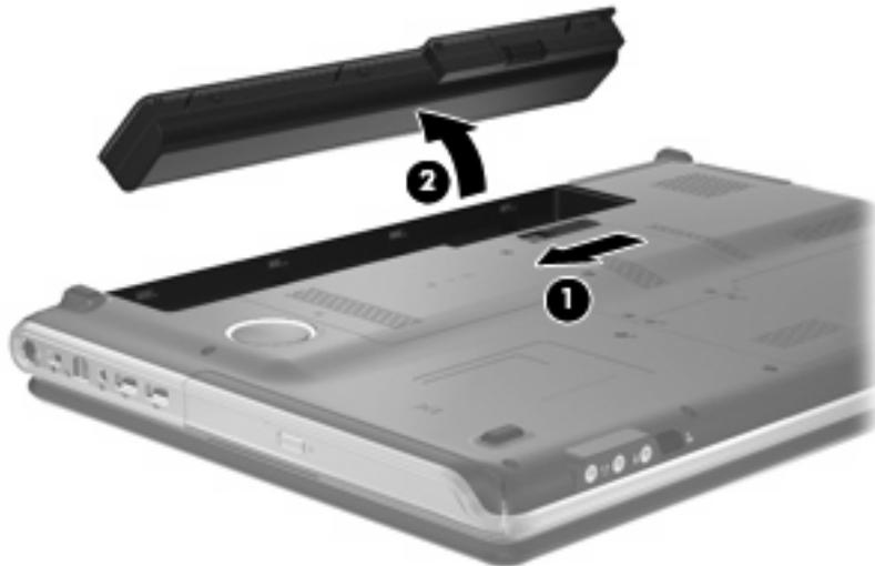
To insert the battery, insert the rear edge of the battery into the battery bay and pivot the front edge of the battery downward until it is seated. The battery release latch automatically locks the battery into place.
