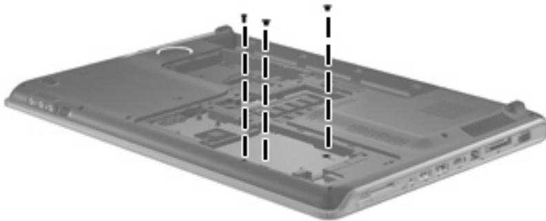
**Where used:** 3 screws, located inside the hard drive bay, that secure the top cover to the computer
