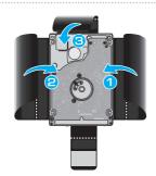
Fold the Mylar as shown in the picture and ensure that the Mylar covers the HDD from all sides.
