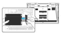
Open the back cover of the laptop and connect the SATA Bus with HDD/SSD.
