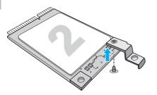
Fasten the mSATA bracket onto the 2nd mSATA SSD as shown.
