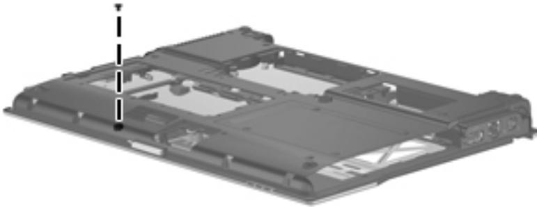
**Where used:** One screw that secures the top cover to the base enclosure
