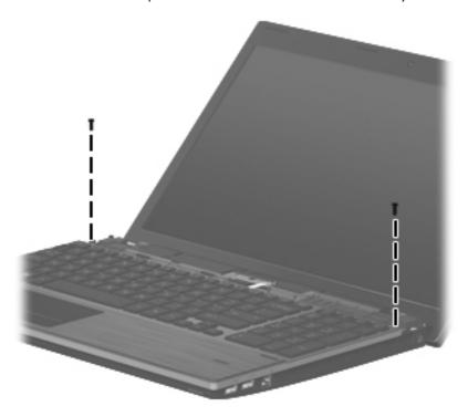
**6.** Slide the keyboard back toward the display **(1)**, and then rotate it forward **(2)** until it rests upsidedown on the palm rest.
