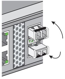
**4.** Insert the fiber optic cables into the installed transceivers.
