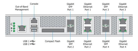
The RFS7010 RF Switch has four RJ-45 Gigabit Ethernet ports, four Gigabit SFP (fiber) ports, one Outof-band management port and one Console connector. The above diagram shows each of those ports and the cables or devices attached to them. The sections that follow describe detailed connection and cabling information for each port. For software configuration, please see the RFS7000 Series RF Switch System Reference Guide available from the Motorola website.
