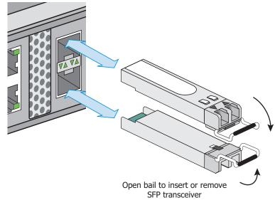
2. Insert each of the SFP transceivers into the corresponding ports on the switch.
