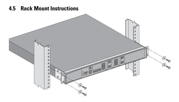
To install the RFS7000 Series RF Switch in a rack:
