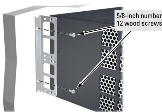
Figure 2-13. Installing wood screws for wall mounting
