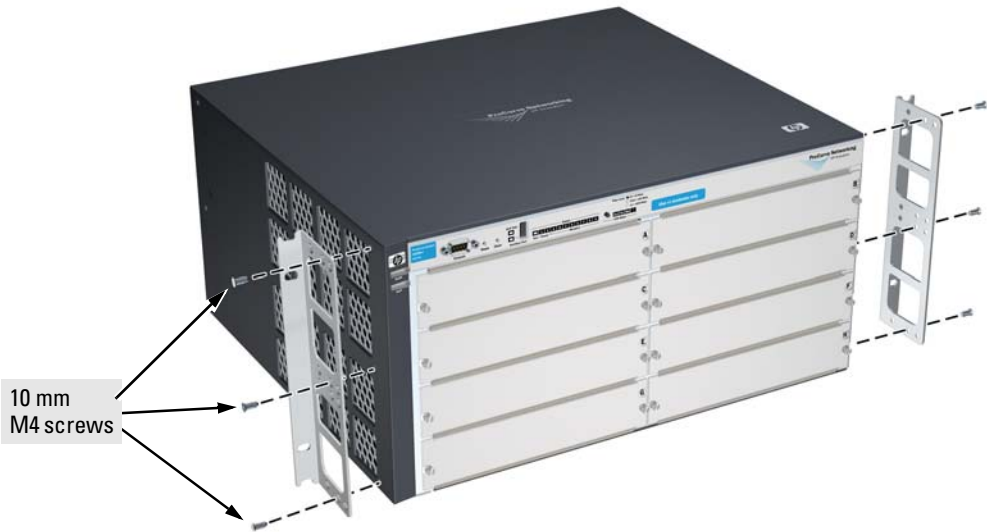
Figure 2-8. Attaching brackets to a 5U chassis
