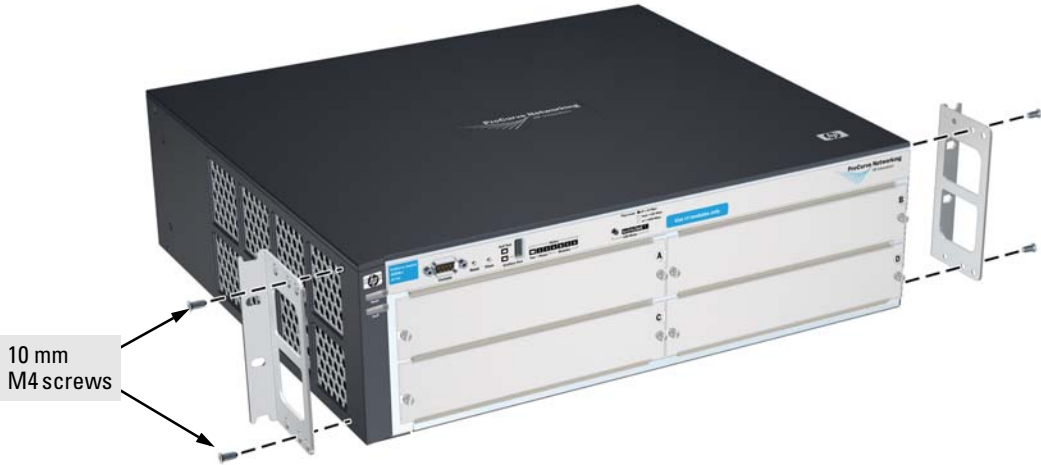
Figure 2-7. Attaching brackets to a 3U chassis
