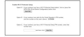
Push button: You may push the WPS button on the web menu or use the physical button on the back of the Smart Repeater.
