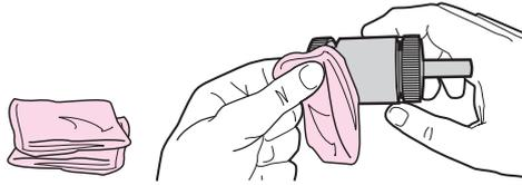
3. Using a dry, lint-free cloth, wipe the pickup roller to remove loosened dirt.
