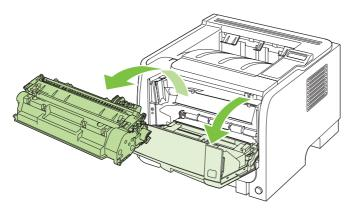
2. Remove the new print cartridge from the bag. Place the used print cartridge in the bag for recycling.
