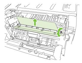
**5.** Replace the print-cartridge, and close the print-cartridge door.
