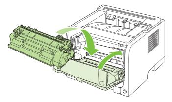
6. Installation is complete. Place the used print cartridge in the box in which the new cartridge arrived. See the enclosed recycling guide for recycling instructions.
