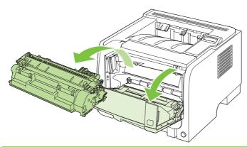
△ CAUTION: To prevent damage, do not expose the print cartridge to light. Cover it with a piece of paper.
