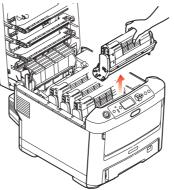
**4.** Put the assembly down gently onto a piece of paper to prevent toner from marking your furniture and to avoid damaging the green drum surface.
