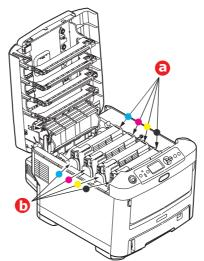
**3.** Holding it by its top centre, lift the image drum, complete with its toner cartridge, up and out of the printer.
