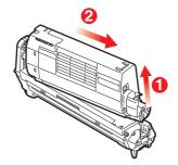
**7.** Take the new image drum cartridge out of its packaging and place it on the piece of paper where the old cartridge was placed. Keep it the same way round as the old unit. Pack the old cartridge inside the packaging material for disposal.
