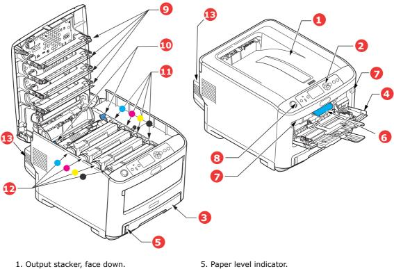
Standard printed copy delivery point. Holds up to 250 sheets at 80g/m<sup>2</sup>.
