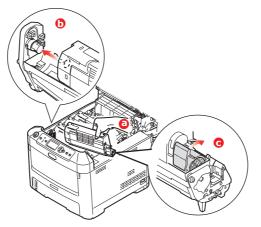
**10.** Pressing gently down on the cartridge to ensure that it is firmly seated, push the coloured lever towards the rear of the printer. This will lock the cartridge into place and release toner into the image drum unit.
