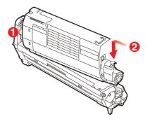
**9.** Push the coloured release lever away from you to lock the toner cartridge onto the new image drum unit and release toner into it.
