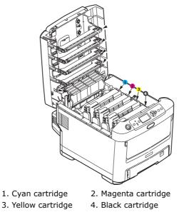
(a) Pull the coloured toner release lever on the cartridge to be replaced fully towards the front of the printer.
