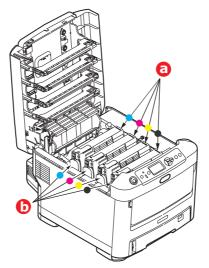
**3.** Lift each of the image drum units out of the printer and place them in a safe place away from direct sources of heat and light.
