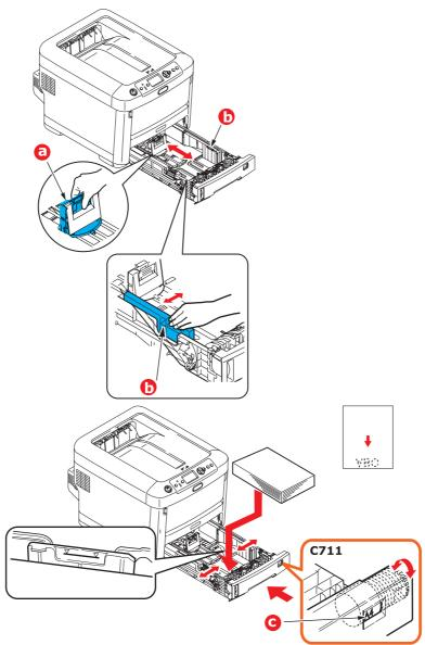
> Adjust the rear stopper (a) and paper guides (b) to the size of paper being used.
