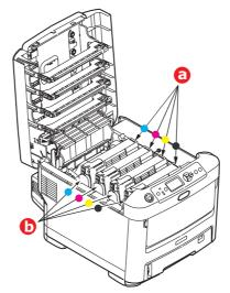
It will be necessary to remove the four image drums to gain access to the paper path.
