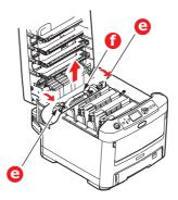
(e) Press release lever (g) and pull the trapped paper from the fuser.
