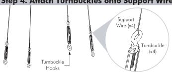
Loop each dangling Support Wire through a Turnbuckle, and wrap 5 times to secure.
