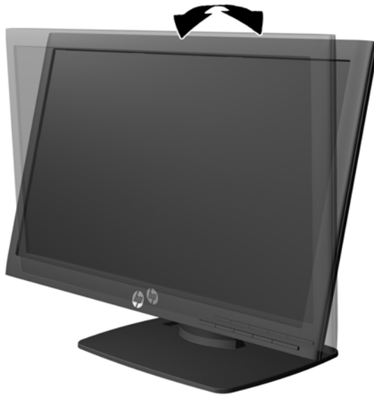
Figure 2-4 Tilting the Monitor
