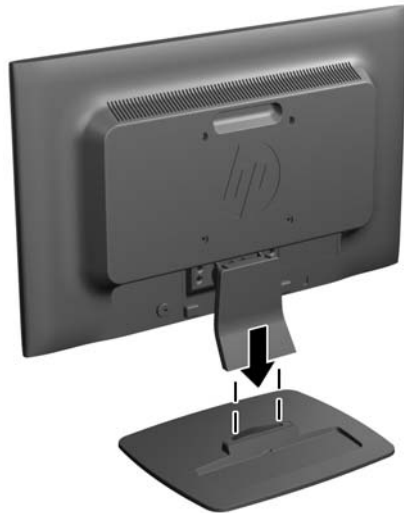
Figure 2-1 Attaching the Monitor Base
