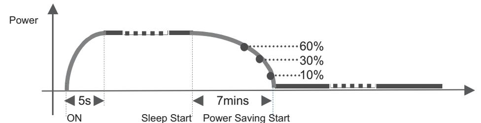
This “Slow-Start-n-Delay-Off” approach minimizes the transit of electricity and temperature caused by the turn-on and turn-off of LCD monitor. Therefore, the decay of backlights of TFT-LCD can be controlled in the certain level which is much less than it was.
