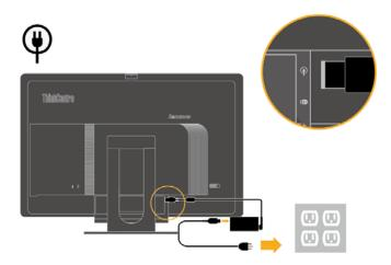
4. Connect one end of the power cord of the external desktop computer to the computer and the other end to a properly-grounded electrical outlet.
