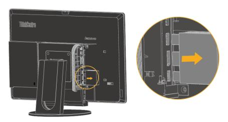
2. Remove the screw that secures the computer.
