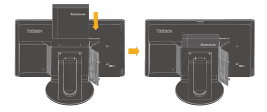
3. Press the top of the computer to insert it into the bay completely.
