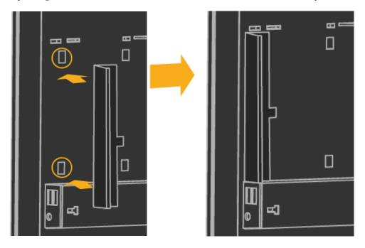
5. Pivot the optical drive bay cover as shown to the closed position.
