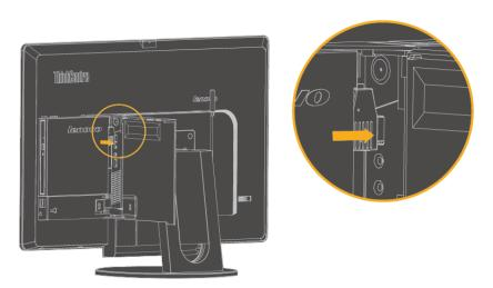
4. Insert the four hooks into the corresponding holes in the optical drive bay as shown. Then, move the optical drive rightward a bit to make the four hooks secured by the holes.
