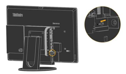
5. Slide the 3-in-1 cable to the left to connect it to the corresponding connectors on the computer. From top to bottom, they are USB connector, DisplayPort connector, and ac power adapter connector.
