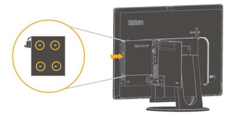
5. Pivot the optical drive bay cover as shown to the closed position.
