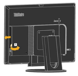
3. Disconnect the optical drive cable from the USB connector on the computer. Then, remove the optical drive from the bay.
