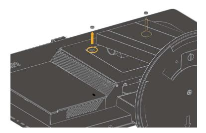
3. Remove two screws covered by the two rubber cushions. Then, remove the full-function monitor stand.
