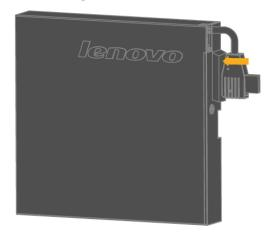
3. Carefully align and manually insert the optical drive cable into the USB connector on the Tiny as shown.
