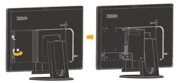
2. Pull out the optical drive cable, and then locate the connector in the holder as shown.
