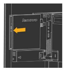
4. If the decorative cover of the optical drive bay is available, insert the two tabs on the cover to the corresponding holes in the monitor. Ensure that the decorative cover is secured firmly.
