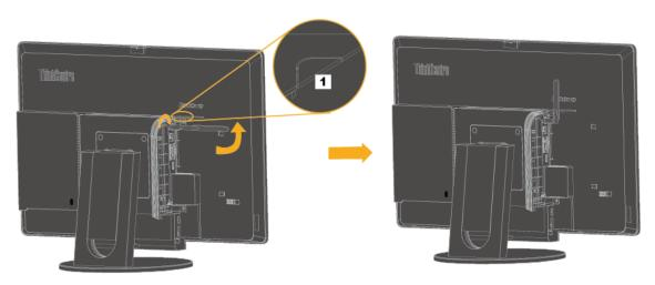
2. Pivot the cable cover as shown to the closed position.
