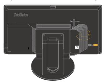
2. Pivot the rear Wi-Fi antenna downward at an angle of about 90°. Then, hold the thicker end of the rear Wi-Fi antenna and unscrew it from the computer.
