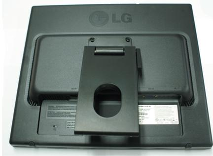
2. Separate the head and the stand with the use of a screwdriver.
