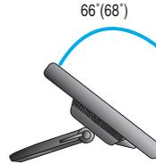
■ Push back the panel to the end, and use from the point that it automatically returns.
