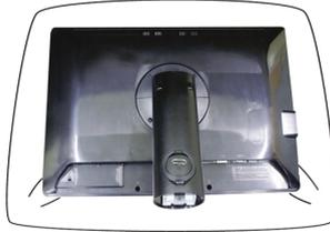
2. Align the hooks on the Stand Body with the matching slots in the Stand Base.
