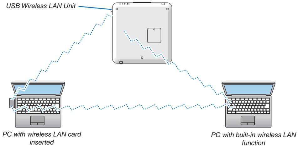
To enable direct communication (i.e., peer-to-peer) between computers and projectors, you need to select the Ad Hoc mode. (→ page 136)
