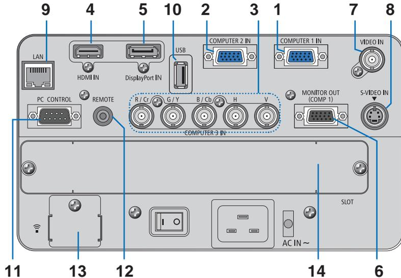
1. **COMPUTER 1 IN / Component Input Connector (Mini D-Sub 15 Pin)** (→ page [13](#), [156](#), [161](#))
