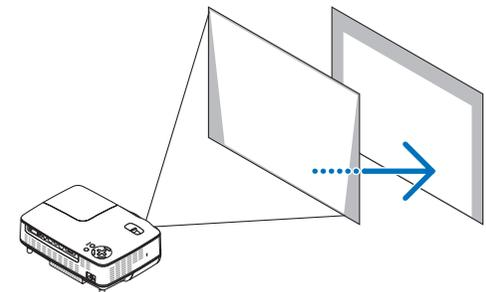
**TIP:** If the projected image is distorted horizontally, move the projector left or right to center the image horizontally on the screen.
