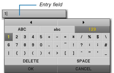
**5. After completing entry, press the ▼ button and move the cursor to select [OK] and the ENTER button.**
