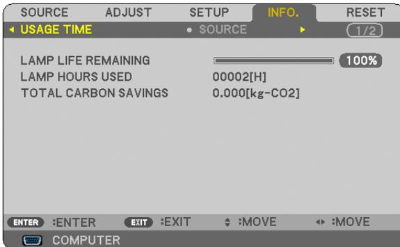
The [CARBON SAVINGS-SESSION] message shows the amount of CO<sub>2</sub> emission reduction between the time of changing to ECO MODE immediately after the time of power-on and the time of power-off. The [CARBON SAVINGS-SESSION] message will be displayed in the [POWER OFF/ ARE YOU SURE?] message at the time of power-off.
