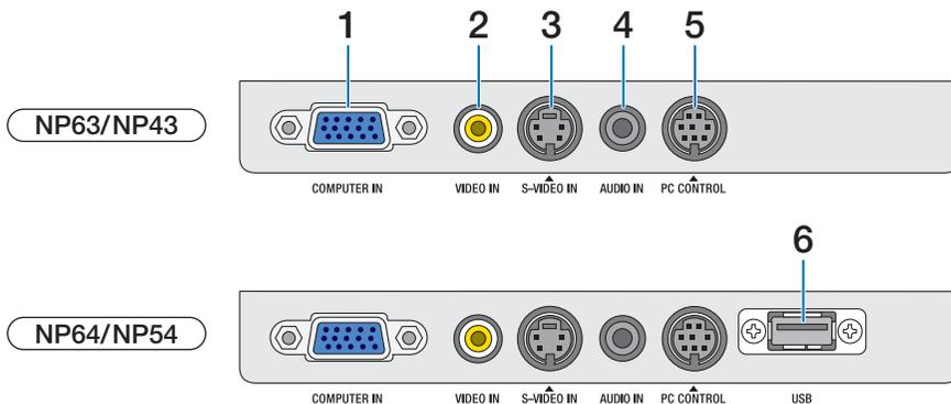
1. **COMPUTER IN/ Component Input Connector (Mini D-Sub 15 Pin)** (→ page 12, 13)
