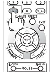
If the projector can be operated with the current remote control ID, the [ACTIVE] will be displayed. If the projector cannot be operated with the current remote control ID, the [INACTIVE] will be displayed. To operate the inactive projector, assign the control ID used for the projector by using the following procedure (Step 3).
