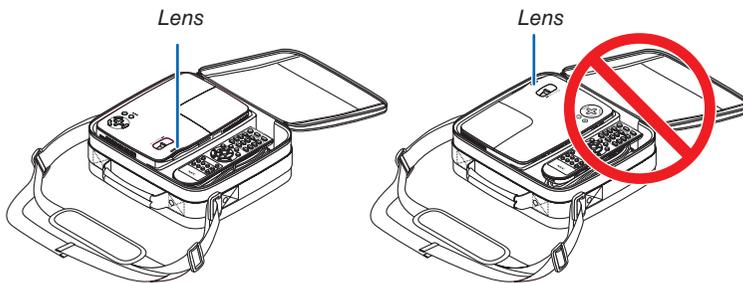
*NOTE: When placing the projector in the soft case, retract the tilt foot and the rear feet. Failure to do so may cause damage to the projector.*
