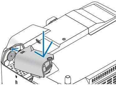
(2) Tighten the cooling pump cover screw.
