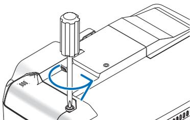
(2) Remove the cooling pump cover.
