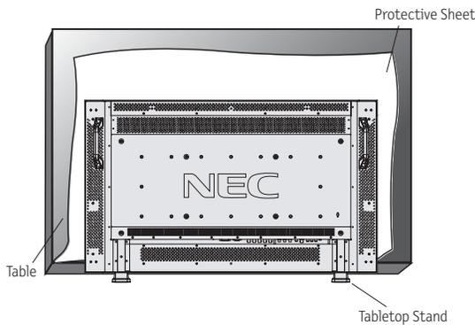
To avoid damaging the screen face, place the protective sheet on the table underneath the LCD. The protective sheet was wrapped around the LCD in the original packaging. Make sure there is nothing on the table that can damage the monitor.
