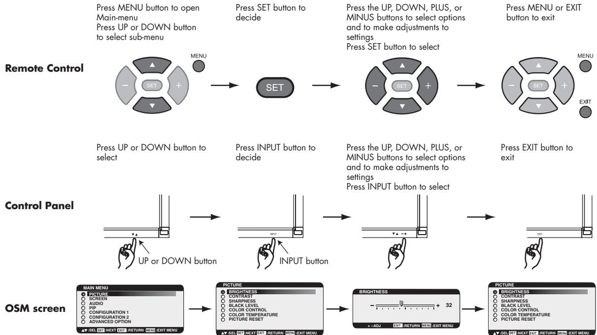
**NOTE:** Items in this OSM menu may change depending on connection type and with the AV unit installed.
