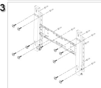
Check the installation diagram and mark the drill points on the wall. Use the 5.0 mm bit to drill holes deeper than 35 mm. Fix each anchor in the corresponding hole.
