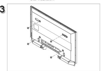
Tighten the 4 screws in step 2 (plastic hanger + screw B)to the rear holes of the product.
