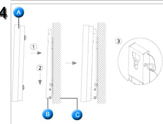
Remove safety pin (3) and insert the 4 product holders into the corresponding bracket holes (1). Then place the product(2) so that it is firmly fixed to the bracket. Make sure to re-insert and tighten the safety pin (3) to securely hold the product to the bracket.
