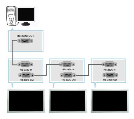
A Multiple Display Control (MDC) is an application allowing various displays to be easily and simultaneously operated on a PC. RS-232C, a standard of serial communication, is used for the communication between a PC and a display. Therefore, a serial cable should be connected between the serial port on a PC and the serial port on a display.
