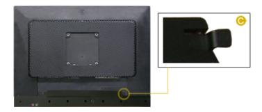
For removal, push and lift up part ( ) towards the inside and remove it. Failing to do so may damage the unit.
