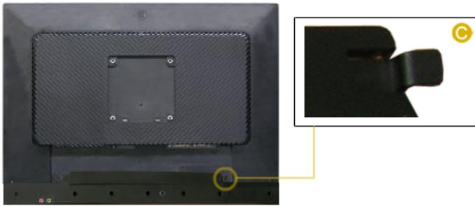
For removal, push and lift up part (C) towards the inside and remove it. Failing to do so may damage the unit.
