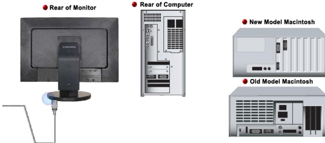
1. Connect the power cord for your monitor to the power port on the back of the monitor. Plug the power cord for the monitor into a nearby outlet.
