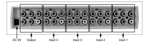
**NOTE:** These instructions assume that all devices connected to the switch use the same connection that the switch will use to connect to the display (i.e. the switch connects to the Component Video input on a television, so all devices will be connected to the switch using Component Video cables).
