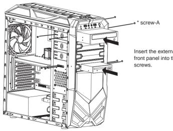
Insert the external 5.25" & 3.5" device from the front panel into the chassis then secure with screws.
