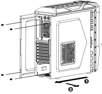
Unscrew to remove left and right panels.
