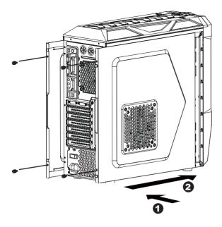
Make sure all necessary cables and wires are connected, then reinstall side panels and secure with screws.
