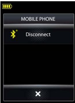
2. Touch **Disconnect**. This causes the base (and also the headset) to disconnect the mobile phone, indicated by greyed out target icon with the Bluetooth® icon. See figure left.
