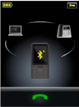
3. Touch the Bluetooth® button on the mobile phone icon. This causes the base to start reconnecting to the mobile phone, indicated by the flashing Bluetooth® icon. See figure left.
