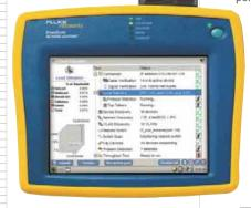
Fluke's EtherScope automatically scans wireless LAN channels.
