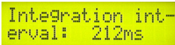
Fig. 14: Setting the integration interval, this is the time the DSP evaluates the signal to establish whether it should respond or not
