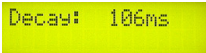
Fig. 13: Setting the decay time, this is the time the compressor needs to respond after the input signal falls back to normal level (below threshold).
