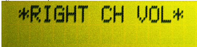
Fig. 16: Changing right input channel gain
