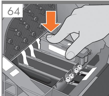
**EN** Push each printhead into the slot until it clicks into place. The front panel tells you whether the printhead has been inserted correctly.
