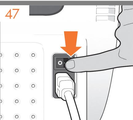
**EN** Switch on power to the product using the switch just above the power socket. Remove the plastic film covering the window and the plastic film covering the front panel (LCD display).
