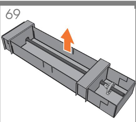
**EN** **Media load for T790 & upper roll in T1300** When the front panel prompts you to load paper for printhead alignment: Take the spindle which comes in a separate box, and use it to load the paper the first time.
