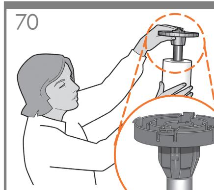
If the blue removable stop is on the spindle, remove it. Put the roll onto the spindle, making sure to put it on the right way round: the leading edge of the paper should go into the product from the top of the roll. Add the removable stop to the spindle to keep the roll in place.
