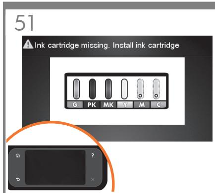
The product checks for the presence of ink cartridges. On finding none, it prompts you to install the ink cartridges.
