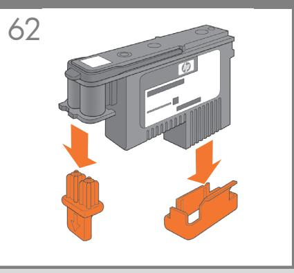
**EN** Unwrap each printhead and remove all orange parts.
