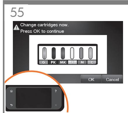
**EN** When you have inserted all of the ink cartridges correctly, the product must prepare the ink system for its first use. It will do this immediately if you press the OK key, or after a 60-second pause if you do not press the OK key. When the ink system is ready, the front panel will prompt you to open the window.
