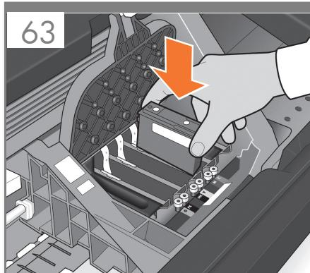
**EN** Insert the printheads one by one. Each printhead is marked with its own colors, and should be inserted only into the correct slot marked with the same colors. Insert the printheads with the blue handle towards you.
