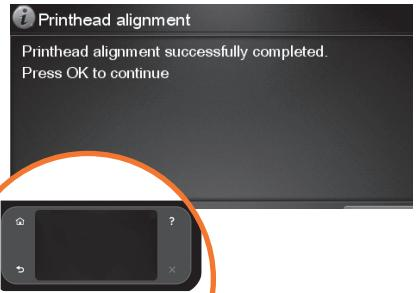
**EN** The front panel will display a series of messages showing the progress of the printhead alignment. There is no need to take any action until the alignment has finished, when you will see the message shown below. Press the OK key.
