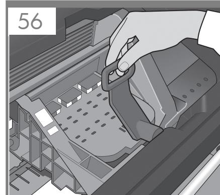
**EN** Open the window and grasp the blue handle of the printhead cover.
