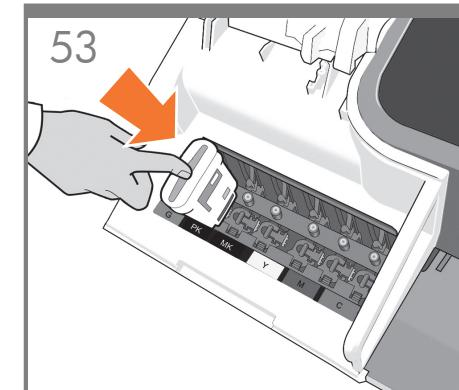
Insert the ink cartridges one by one. Each cartridge is marked with its own color, and should be inserted only into the slot of the same color. Avoid touching pins, leads or circuits.
