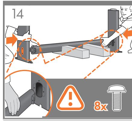
**EN** Attach each leg of the stand to the cross-brace, using two screws **on the outside** of the leg and then two **on the inside**. First fit all four screws loosely, then tighten up the screws **on the outside** of the leg, followed by the screws **on the inside**.
