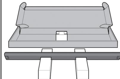
Place the two pieces of packaging material on the floor, spaced 40 cm apart, and place the cross-brace on top of them.
