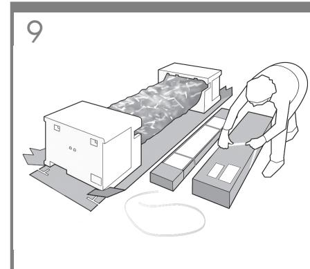
**EN** Cut and remove the straps around the stand box. **Do not remove the white protective material until instructed to do so.**
