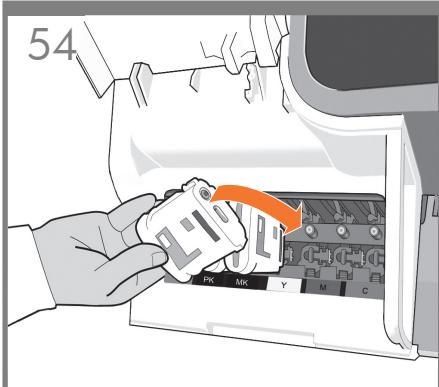
**EN** The cartridges must be inserted the right way around: the ink outlet in the cartridge should meet the ink inlet in the slot. Push the cartridge into the slot until it clicks into place. The product beeps whenever a cartridge is successfully inserted.
