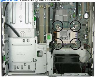
When reinstalling the heatsink, make sure that its bottom has been cleaned with an alcohol wipe and fresh thermal grease has been applied to the top of the processor.
