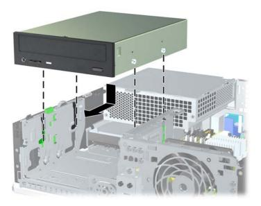
Rotate the drive cage to its upright position.
