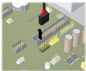
Figure 7-27 Disconnecting the Media Card Reader 1394 Cable
