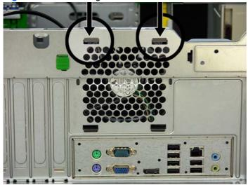
To install the fan assembly, insert the bottom tabs into the slots in the chassis, and then rotate the fan upward until the top tabs snap into place. Be sure to orient the air flow out of the unit.
