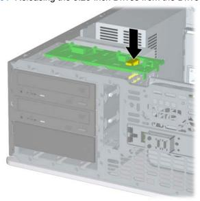
Before you reinstall each drive into the chassis, turn it so that it is in the same orientation as the internal 3.5-inch drive. The bottom of the drive should be parallel to the yellow drivelock.
