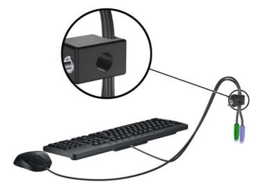
Screw the lock to the chassis using the screw provided.
