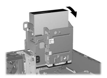
6. Press down on the green drive retainer button located on the left side of the drive to disengage the drive from the drive cage (1). While pressing the drive retainer button, slide the drive back until it stops, then lift it up and out of the drive cage (2).
