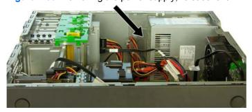
Slide the power supply toward the front of the computer, rotate toward the fan so the power supply clears the lip on the top of the chassis, and then lift the power supply out of the chassis.
