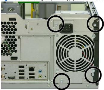
Press the tab in front of the power supply that holds it in place.
