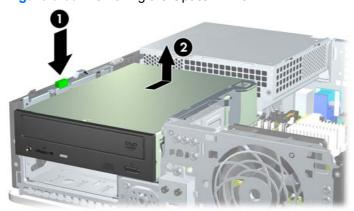
NOTE: To replace the optical drive, reverse the removal procedure. When replacing a drive, transfer the four guide screws from the old drive to the new one.
