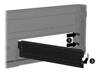
To remove the 5.25-inch bezel blank, push the two retaining tabs that hold the bezel blank in place towards the outer left edge of the bezel (1) and pull the bezel blank inwards to remove it (2).
