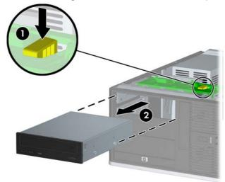
• To remove a 3.5-inch drive or a 5.25-inch drive in the minitower configuration, pull up on the green drivelock mechanism (1) for that specific drive and slide the drive from the drive bay (2).
