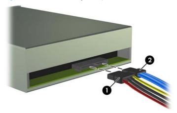
• If you are removing a diskette drive, disconnect the data cable (1) and power cable (2) from the back of the drive.
