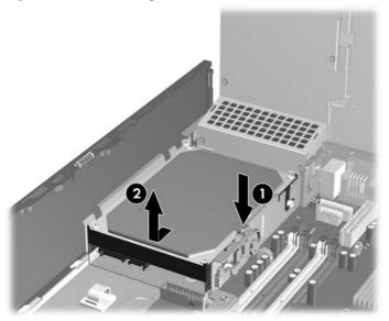
To install a hard drive, you must transfer the silver and blue isolation mounting guide screws from the old hard drive to the new hard drive.
