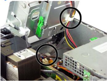
Pull the power supply forward until the posts on the power supply move forward in the power supply bracket, and then lift the power supply straight up and out of the chassis.
