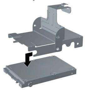
**8.** Transfer the three remaining guide screws (two on the right and one on the rear left) from the old drive to the new drive.
