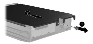
3. Remove the adhesive strip that secures the thermal sensor to the top of the hard drive (1) and move the thermal sensor away from the carrier (2).
