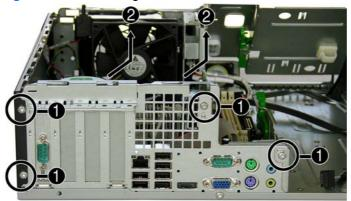
To replace the backwall, reverse the removal procedures.
