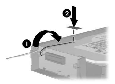
9. Slide the cover on the carrier (1) and replace the screw on the rear of the carrier to secure the cover in place (2).
