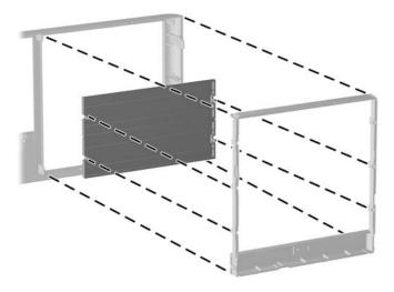
NOTE: When replacing the subpanel, ensure that the aligning pins and any remaining bezel blanks are in their proper orientation. The logo on the subpanel should be located at the bottom of the subpanel when properly oriented.
