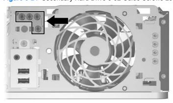
Figure 8-25 Extra Optical Drive M3 Guide Screws Location
