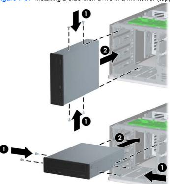
Figure 7-31 Installing a 5.25-Inch Drive in a Minitower (top) and Desktop (bottom)
