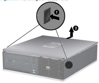
To install the access panel, reverse the removal procedure.
