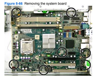
13. Lift up the front of the system board, and then pull the system board forward, up, and out of the chassis.
