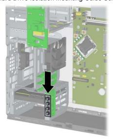
Figure 7-21 Extra Optical Drive M3 Guide Screws Location
