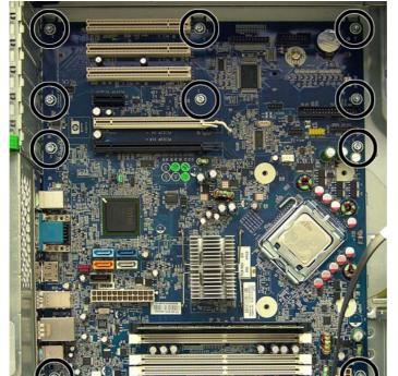
Figure 7-54 Removing the system board
