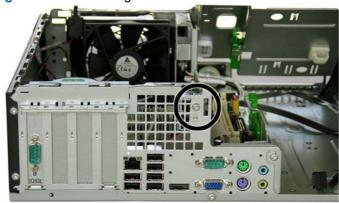
To install the Smart Cover Lock, reverse the removal procedure
