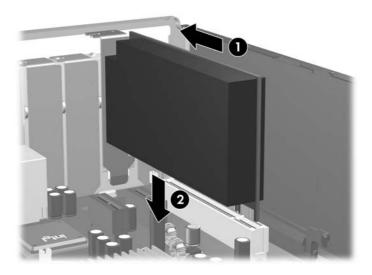
NOTE: When installing an expansion card, press firmly on the card so that the whole connector seats properly in the expansion card slot.
