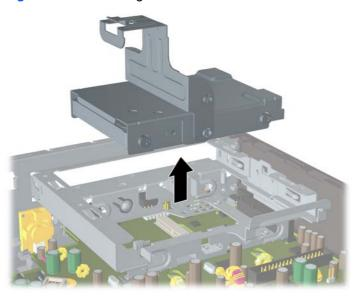
To remove the hard drive from the carrier, remove the guide screw from the front left side of the carrier.
