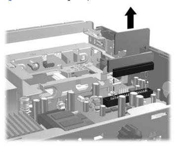
To install the optical drive connector, reverse the removal procedures.
