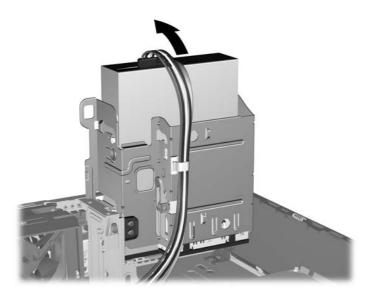
4. Disconnect the power cable (1) and data cable (2) from the rear of the optical drive.
