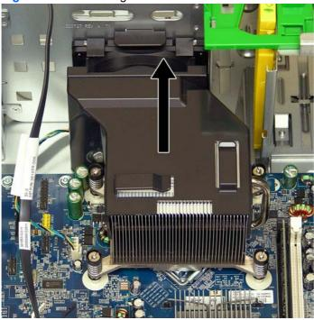
To reinstall the fan shroud, reverse the removal procedure.
