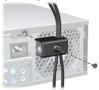
Insert the plug end of the security cable into the lock (1) and push the button in (2) to engage the lock. Use the key provided to disengage the lock.
