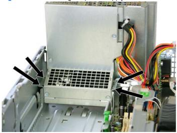
To install the power supply, reverse the removal procedure.
