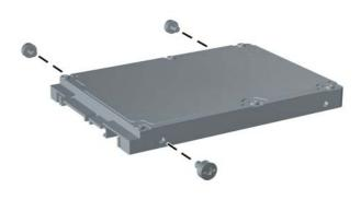
Align the guide screws with the slots on the carrier and slide the new hard drive into the carrier (1), then replace the guide screw on the front left of the carrier to secure the drive in the carrier (2).
