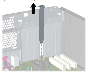
**b.** If you are removing a standard PCI card, hold the card at each end and carefully rock it back and forth until the connectors pull free from the socket. Lift the card straight up to remove it. Be sure not to scrape the card against other components.
