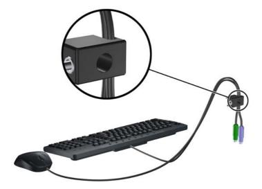
3. Screw the lock to the chassis using the screw provided.
