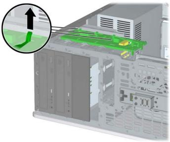
Before you reinstall each drive into the chassis, turn the drive so that it is perpendicular to the internal 3.5-inch drive. The drive should be parallel to the green latch drive bracket.
