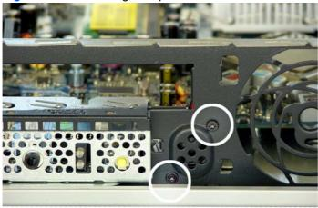
To install the speaker, reverse the removal procedure.
