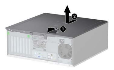
To install the access panel, reverse the removal procedure.
