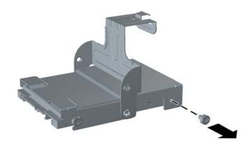
7. Slide the carrier back and remove the hard drive.
