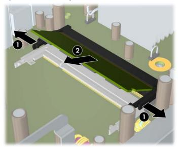
Slide the new SODIMM into the socket at approximately a 30° angle (1) then press the SODIMM down (2) so that the latches lock it in place.
