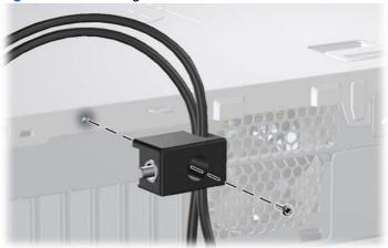
4. Insert the plug end of the security cable into the lock (1) and push the button in (2) to engage the lock. Use the key provided to disengage the lock.
