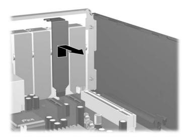
If you are removing a standard PCI card, hold the card at each end, and carefully rock it back and forth until the connectors pull free from the socket. Pull the expansion card straight up from the socket then away from the inside of the chassis to release it from the chassis frame. Be sure not to scrape the card against the other components.
