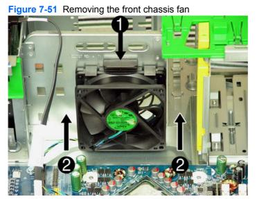
To install the fan assembly, insert the fan tabs into the slots in the inner chassis wall and slide the fan down until it clicks into place. Be sure to orient the air flow out of the unit. Refer to the air flow arrows on the side of the fan housing for proper air flow orientation.
