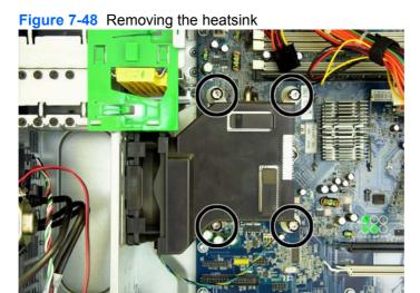
When reinstalling the heatsink, make sure that its bottom has been cleaned with an alcohol wipe and fresh thermal grease has been applied to the top of the processor.
