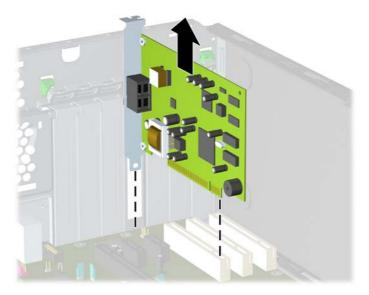
c. If you are removing a PCI Express x16 card, pull the retention arm on the back of the expansion socket away from the card and carefully rock the card back and forth until the connectors pull free from the socket. Lift the card straight up to remove it. Be sure not to scrape the card against other components.
