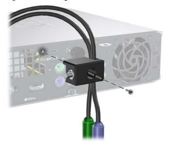
Insert the plug end of the security cable into the lock (1) and push the button in (2) to engage the lock. Use the key provided to disengage the lock.
