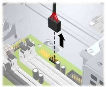
Figure 8-38 Disconnecting the Media Card Reader 1394 Cable
