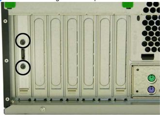
To install the eSATA port, reverse the removal procedure.
