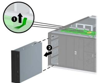
• To remove a hard drive from and internal 3.5-inch drive bay, pull up on the green hard drive drivelock mechanism (1) for that drive and slide the drive from the drive bay (2).
