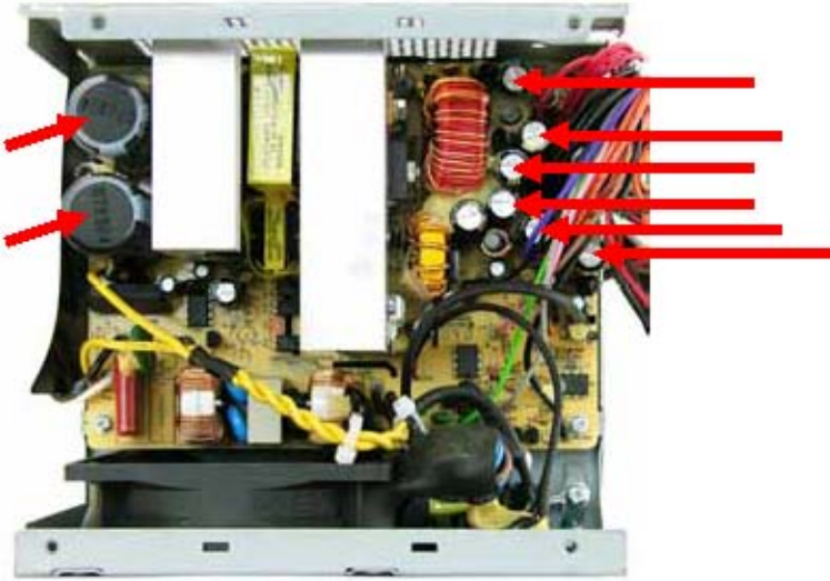
FIGURE 11: Power supply capacitors (8) to cut
