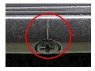
Products affected with defect will have small cracks in the Monitor cover adjacent to the Monitor cover screws at the location shown in the photo.
