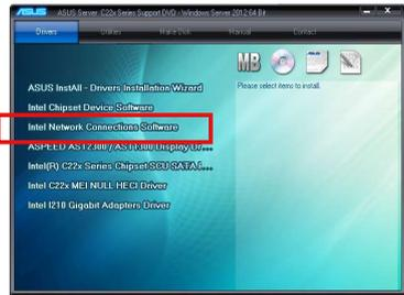
5. From the **Intel® Network Connections** window, click **Install Drivers and Software**.
