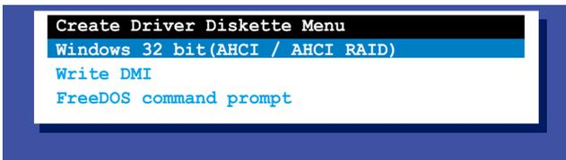
7. From the C22x Intel RAID Driver sub-menu, use the Up or Down arrow keys to select the driver and press <Enter> to create the RAID driver disk.
