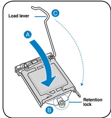
6. Insert the load lever under the retention tab to remove the PnP cap from the CPU socket.
