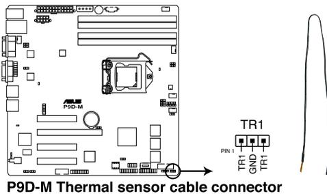
**P9D-M Thermal sensor cable connector**
