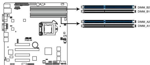
**P9D-M 240-pin DDR3 DIMM sockets**
