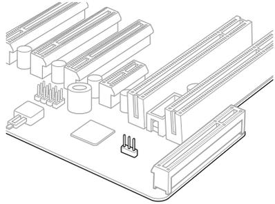
2. Connect the Thermal Sensor cable to the connector.
