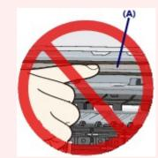
If the paper or your hands touch the clear film and blot or scratch it, the machine can be damaged.
