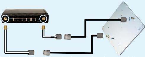
Directional Antennas provide strong coverage for point-to-point solutions. Not recommended for mulitple directional coverage. Please check the antenna specifications to make sure you are selecting the right antenna type for your network environment. Shown above is the Hawking Model # HAO17SDP. For more antenna selection, visit <a href="http://hawkingtech.com/products/178-antennas.html">http://hawkingtech.com/products/178-antennas.html</a>
